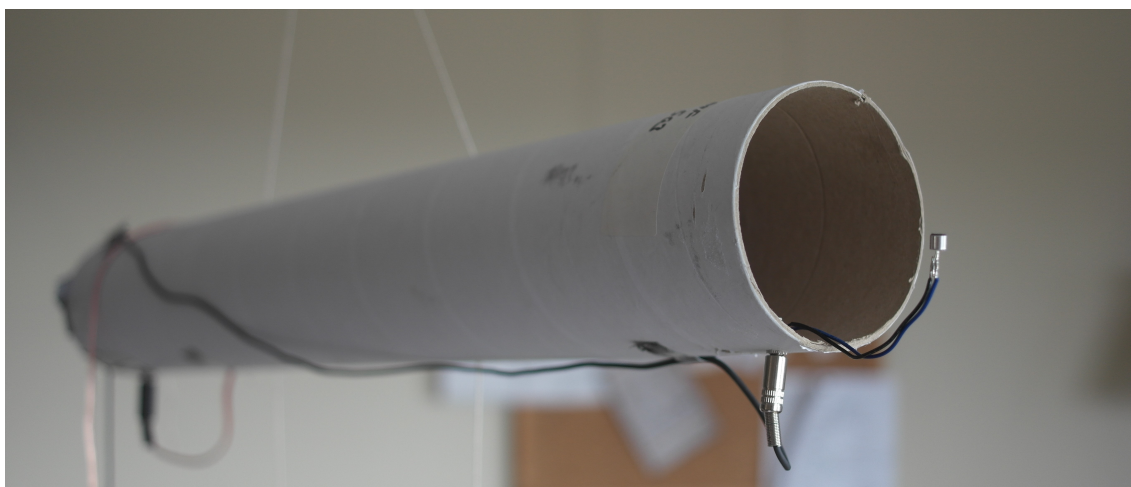
Figure 4.3: Pipe module microphone placement.
